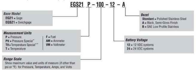
**NOTE:** EG21 and EGS21 are designed for use with 12-volt systems. For 24-volt systems, voltage reducing resistors are included in the wire/connector assembly. No designator required for Standard configurations.
